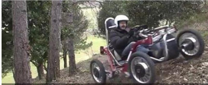
**When riding on a bank, the car remains vertical regardless of the tilt of the wheels.**
